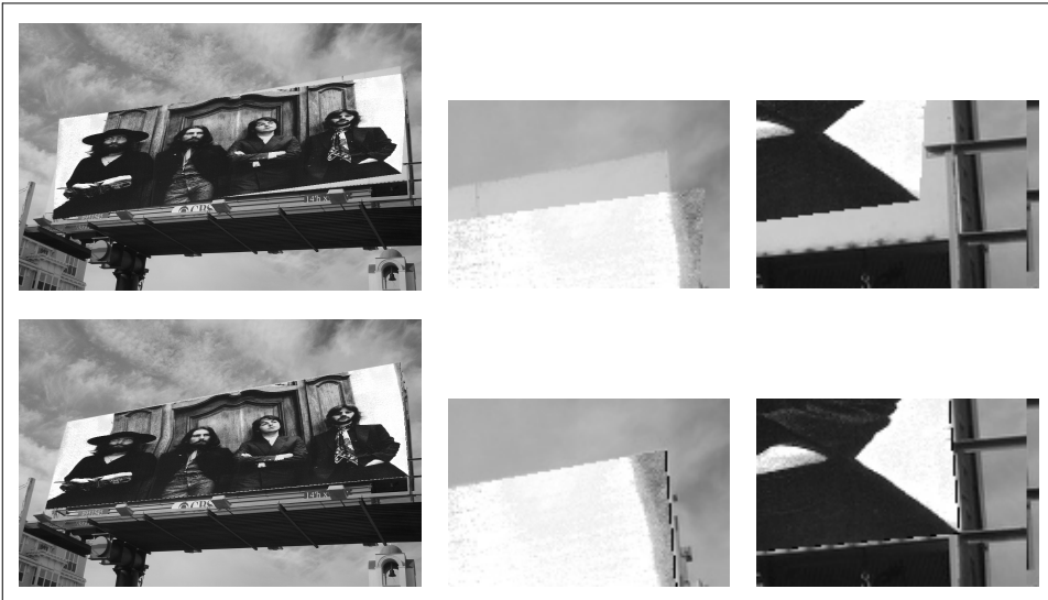
Figure 3-3. Comparing an affine warp of the full image with an affine warp using two triangles. The image is placed on a billboard with some perspective effects. Using an affine transform for the whole image results in a bad fit. The two right-hand corners are enlarged for clarity (top). Using an affine warp consisting of two triangles gives an exact fit (bottom).
