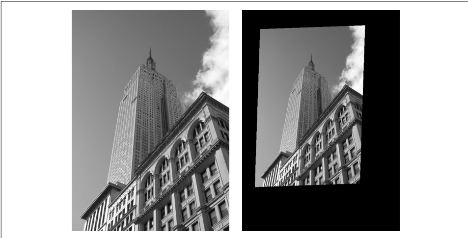
Figure 3-1. An example of warping an image using an affine transform: original (left), image after warping with ndimage.affine_transform() (right).
