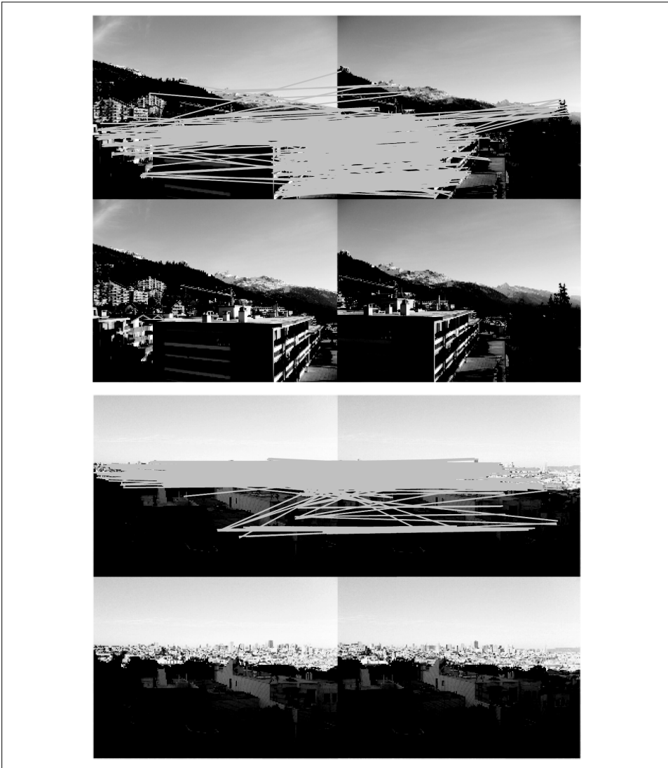
Figure 2-2. Example of matches resulting from applying normalized cross-correlation to patches around Harris corner points.
