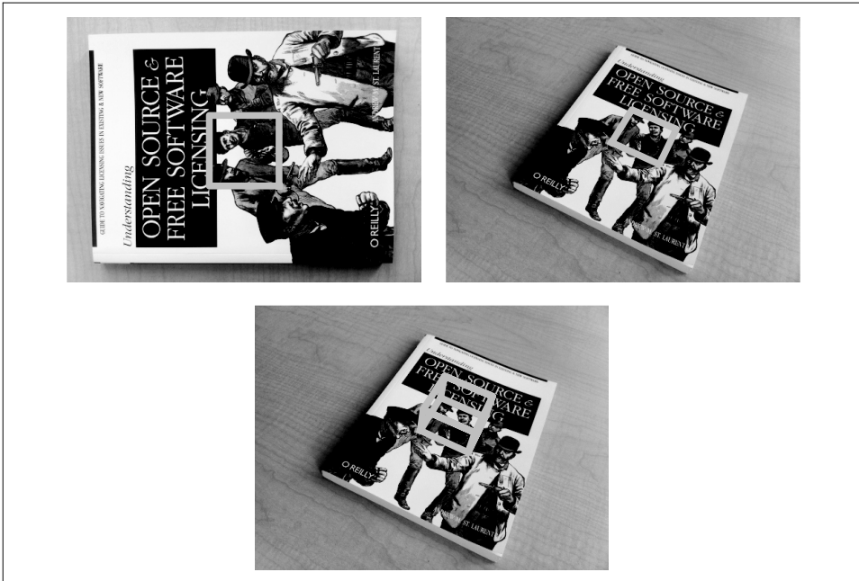
Figure 4-4. Example of computing the projection matrix for a new view using a planar object as marker. Matching image features to an aligned marker gives a homography that can be used to compute the pose of the camera. Template image with a gray square (top left); an image taken from an unknown viewpoint with the same square transformed with the estimated homography (top right); a cube transformed using the estimated camera matrix (bottom).
