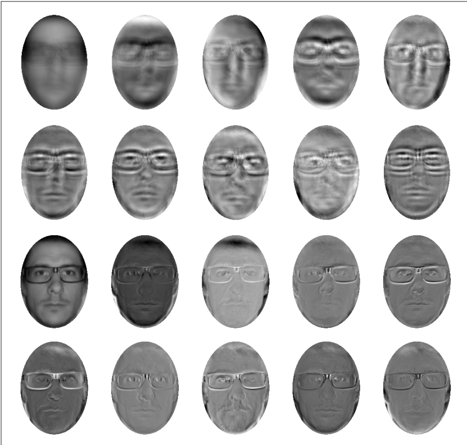
Figure 3-8. Comparing PCA-modes of unregistered and registered images: the mean image and the first nine principal components without registering the images beforehand (top); the same with the registered images (bottom).
