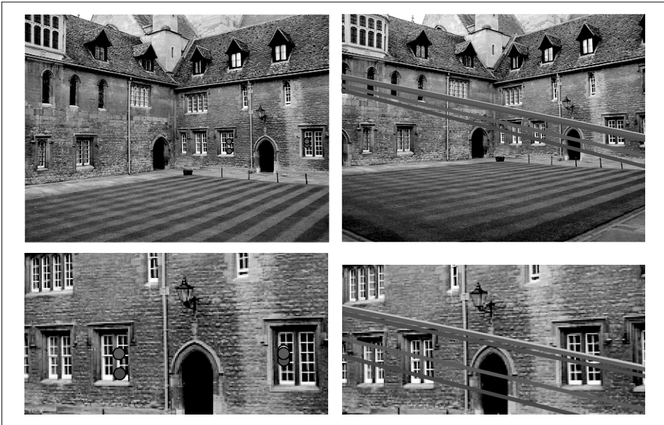
Figure 5-4. Epipolar lines in view 1 shown for five points in view 2 of the Merton1 data. The bottom row shows a closeup of the area around the points. The lines can be seen to converge on a point outside the image to the left. The lines show where point correspondences can be found in the other image (the color coding matches between lines and points).
