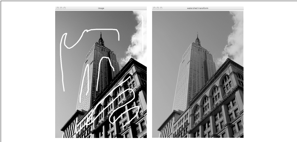
Figure 10-9. An example of segmenting an image using a watershed transform. The left image is the input image with seed regions drawn. The right image shows the resulting segmentation with colors overlaid on the image.
