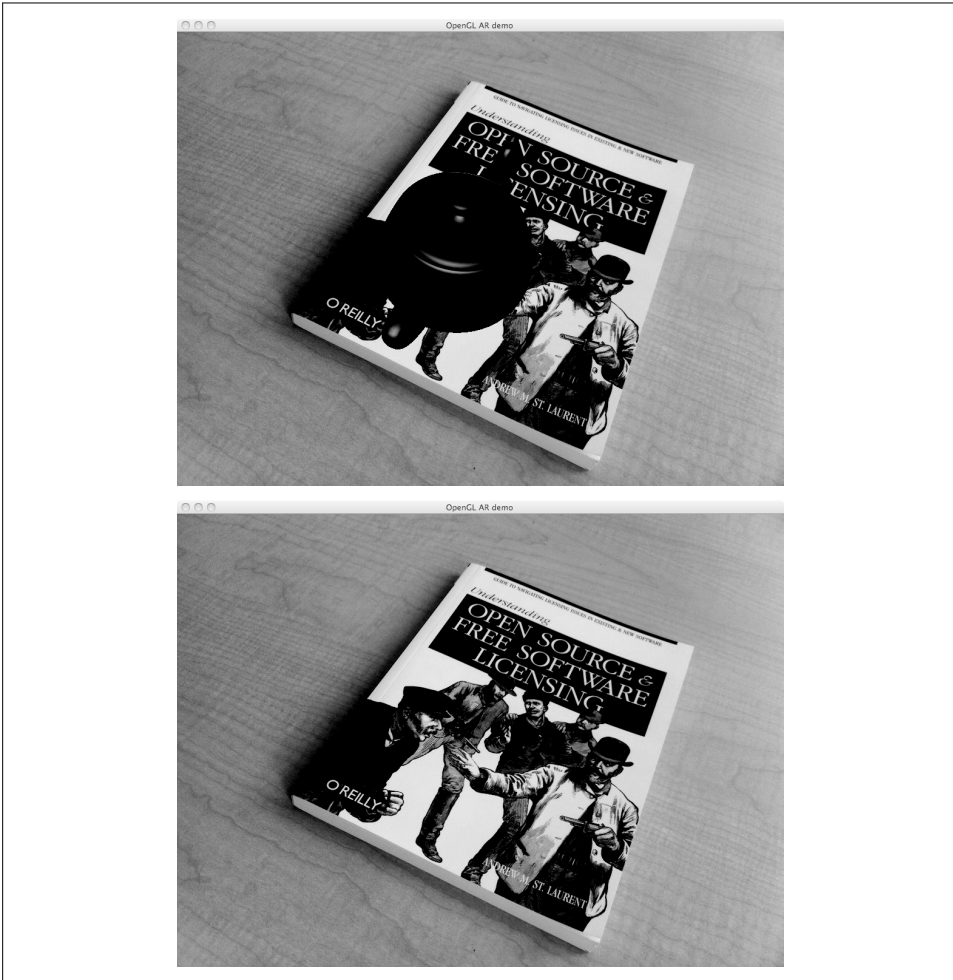
Figure 4-5. Augmented reality. Placing a computer graphics model on a book in a scene using camera parameters computed from feature matches: the Utah teapot rendered in place aligned with the coordinate axis (top); sanity check to see the position of the origin (bottom).
