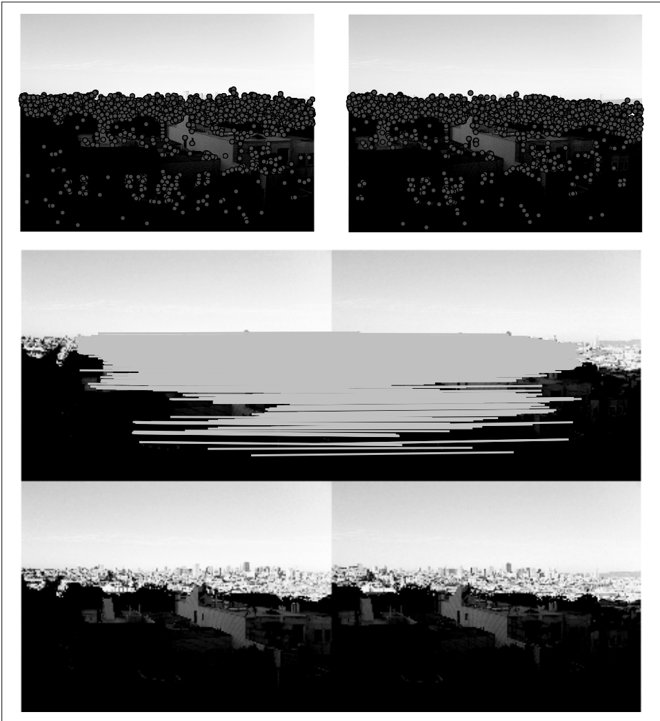
Figure 2-6. An example of detecting and matching SIFT features between two images.
