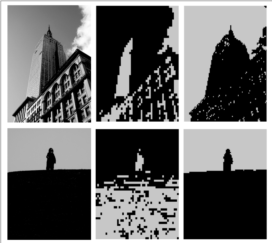
Figure 6-4. Clustering of pixels based on their color value using k -means: original image (left); cluster result with k = 3 and 50 \times 50 resolution (middle); cluster result with k = 3 and 100 \times 100 resolution (right).
