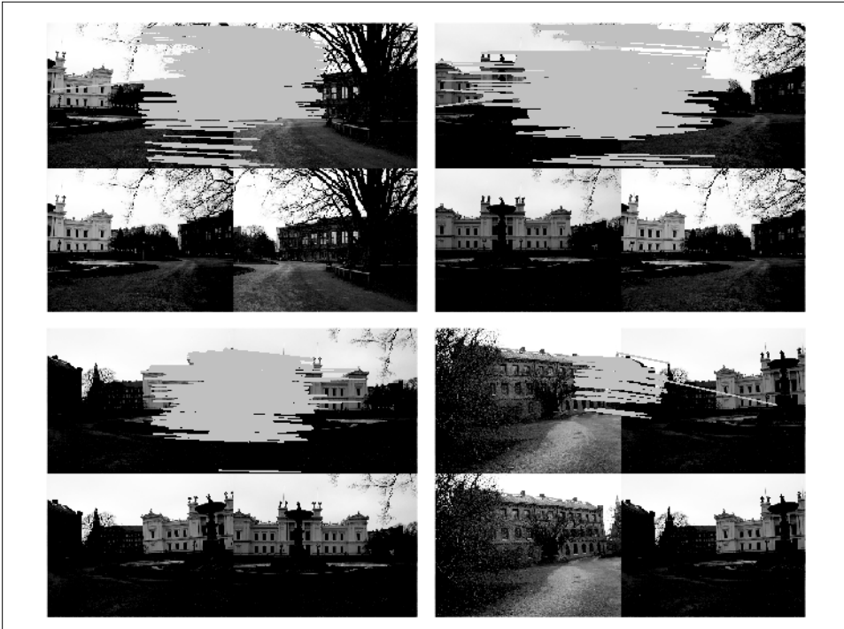
Figure 3-11. Matching correspondences found between consecutive image pairs using SIFT features.
